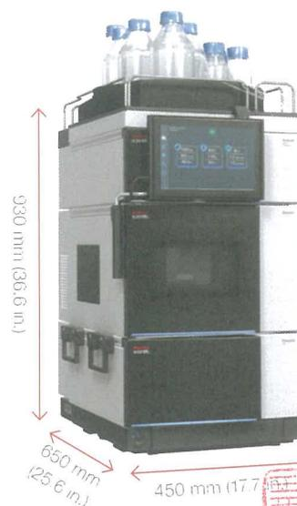
Vanquish Neo UHPLC system with Column Compartment N
