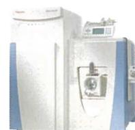
**Thermo Scientific Q Exactive HF hybrid quadrupole-Orbitrap mass spectrometer**
